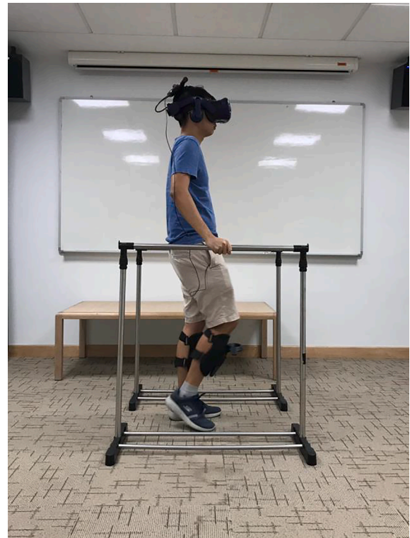
Fig. 3. A researcher wearing the VR headset and wireless controllers on his knees for movement tracking.
